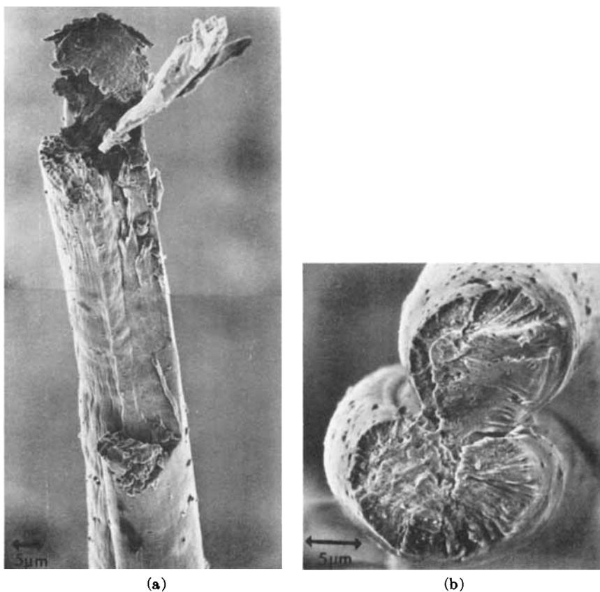
Fig. 11. (a) Orlon Sayelle 21, bicomponent fiber, 0.7 Tex. Tensile break.
