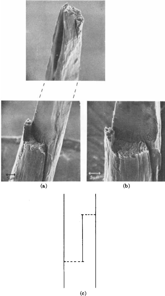
Fig. 5. (a) Courtele, 0.5 Tex, uncrimped tow. Tensile fracture, showing tip and base of split. (b) Courtele 0.5 Tex, uncrimped tow. Tensile fracture, detail of break. (c) Representation of linking of two fractured regions.
