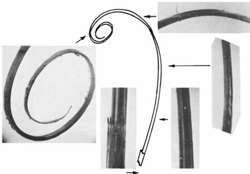
Fig. 15. Courtelle, 1.7 Tex, uncrimped tow, broken in tensile fatigue. Inserts illustrate various sections of the long split region.
