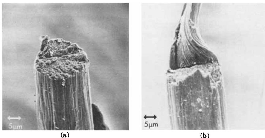
Fig. 7. (a) Courttelle, 0.5 Tex, staple made commercially by the Mackie Process. Tensile fracture perpendicular to fiber axis. (b) Courttelle, 0.5 Tex, staple Mackie Process. Tensile fracture showing fiber splitting up.
