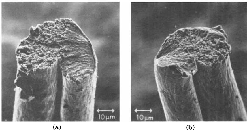
Fig. 9. Opposite ends of Acrilan 1.7 Tex carpet staple, broken in tension.
