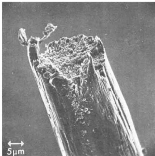
Fig. 1. Courttelle, 0.5 Tex, uncrimped tow. Tensile fracture.
