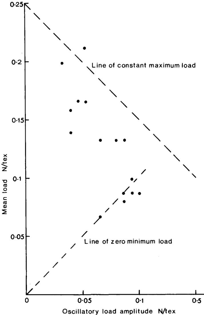
Fig. 12. Failure conditions for tensile fatigue of Courttelle fibers.
