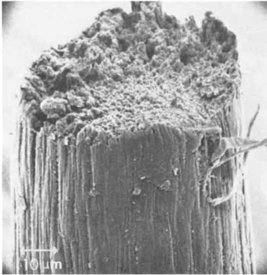
Fig. 3. Courtelle, 1.7 Tex, uncrimped tow. Tensile fracture.
