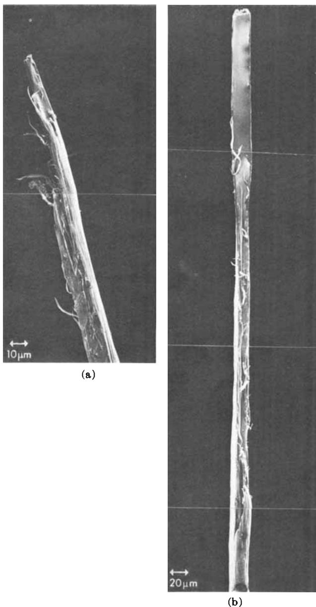
Fig. 6. (a) Courtelle, 0.5 Tex, uncrimped tow. Tensile fracture showing fibrillar end of long split break. (b) Courtelle, 0.5 Tex, uncrimped tow. Opposite end of (a) showing the considerable length of split.
