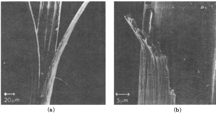
Fig. 16. (a) Courttelle 1.7 Tex, uncrimped tow. Fiber split into three parts during tensile fatigue testing. (b) Courttelle, 1.7 Tex, uncrimped tow, tensile fatigue. Smooth inner surface of split region.
