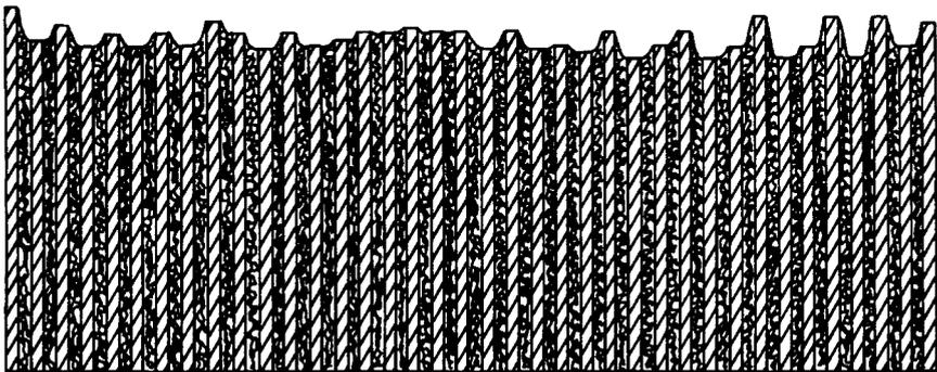
Fig. 4. Schematic representation of acrylic fiber fracture, based on fracture studies of yarns by Monego and Backer.<sup>4</sup>
