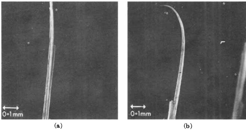
Fig. 13. Opposite ends of Courttelle, 1.7 Tex, uncrimped tow, broken in tensile fatigue.
