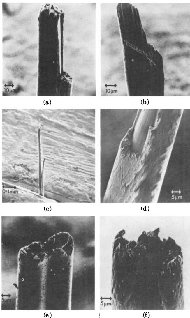
Fig. 10. Tensile fractures of Orlon 42. (a) 0.7 Tex, high bulk staple, split break. (b) 0.7 Tex, crimped tow, split break. (c) 0.7 Tex, Turbo process staple, split break. (d) 0.7 Tex, Turbo process staple, smooth surface in split region. (e) 0.7 Tex, Turbo process staple, break perpendicular to fiber axis. (f) 0.7 Tex, Turbo process staple, rough appearance of fracture surface.
