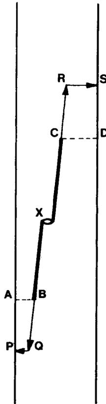
Fig. 14. Schematic representation of nature of axial splitting in fatigue.
