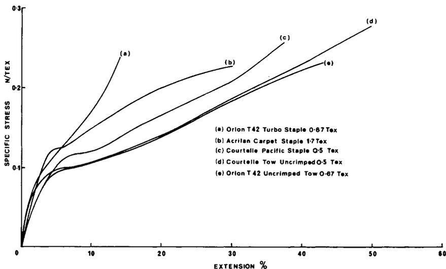
Fig. 2. Stress-strain curves of acrylic fibers.
