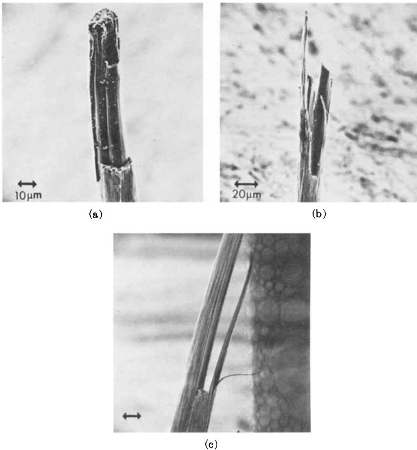
Fig. 8. (a) Courtelle, 0.5 Tex, staple made commercially by Pacific converter. Tensile fracture. (b) Courtelle, 0.5 Tex, staple-Pacific converter. Tensile fracture showing fiber splitting up. (c) Courtelle 1.7 Tex, uncrimped tow. Tensile fracture.
